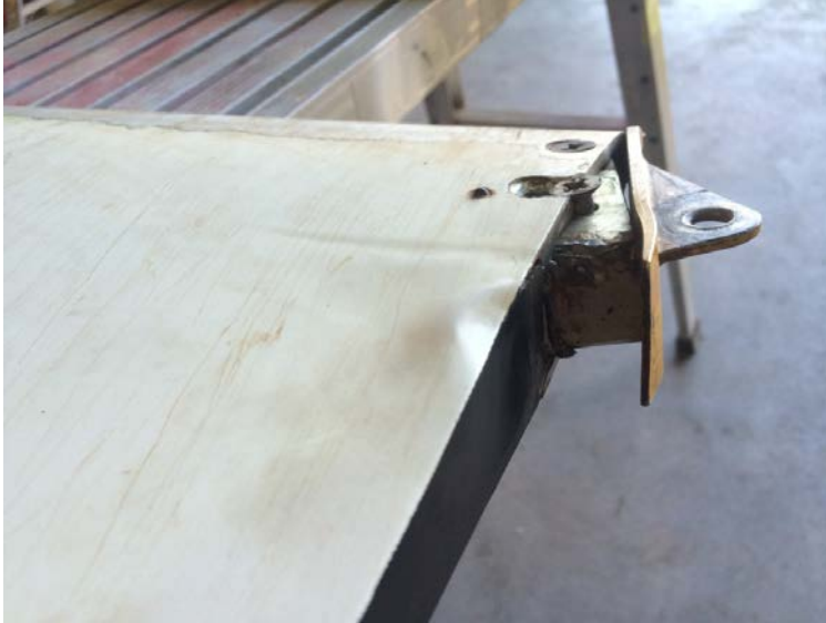
Figure 2: Damage to main rotor blade tip
